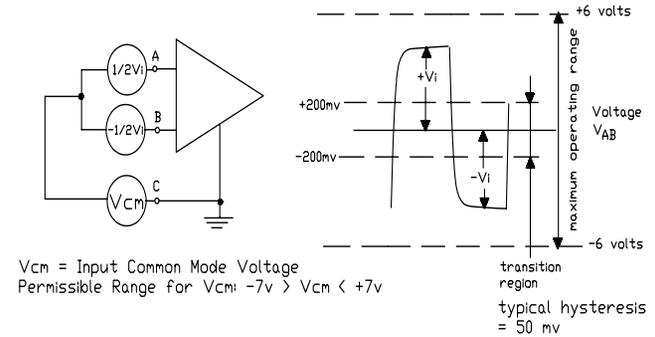
BALANCED DIFFERENTIAL INPUT LINE RECEIVER
