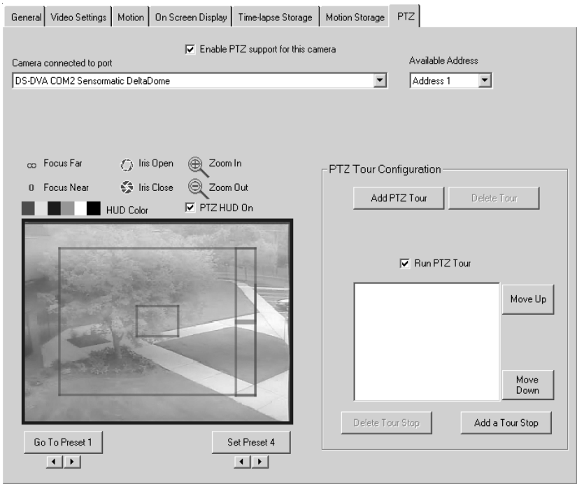
Figure 25 The PTZ tab allows you to configure PTZ cameras, presets, and tours.
