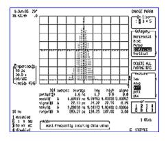
Figure 11 shows the histogram of the period of a 102 MHz sinewave (period equal to 9.804 ns) delivered by a very stable sinewave source. The standard deviation of the period measured shows that the measurement of the period has an RMS repeatability of 27.53 ps. The worst case difference between the smallest measured period and the largest ("range" of the jitter histogram) is 203 ps, representing 2% of the total period value.
