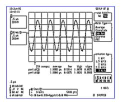
In fact, bandwidth limiting can improve the measurement by reducing noise on the waveform and by allowing the scope to capture more points on a fast signal edge. Note that by applying a 200 MHz filter to the signal edge in Figure 5, the scope can now capture more than two samples on the edge. The 20% to 80% risetime has been slowed to 1.8 ns but the
