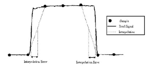
**Width:** Duration between the leading and trailing edges of a pulse waveform as measured between the 50% point on both edges.
