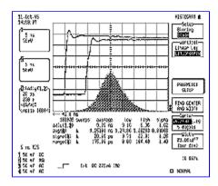
The principal actions for achieving accurate time measurements are: Select the right system bandwidth, minimizing noise but maintaining signal timing fidelity.
