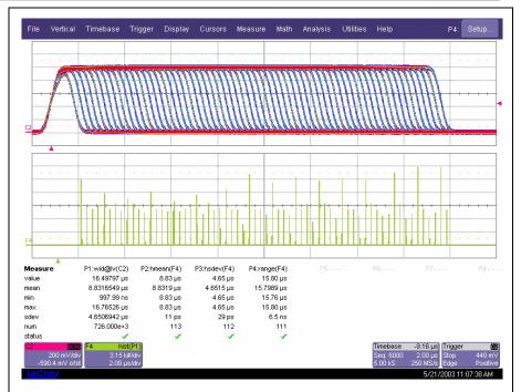
Figure 2 Studying the variation of pulse width using analog persistence
