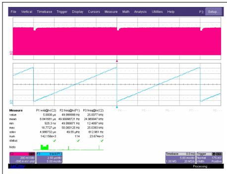
Figure 1 Analyzing a PWM waveform using the track of the width@level parameter
