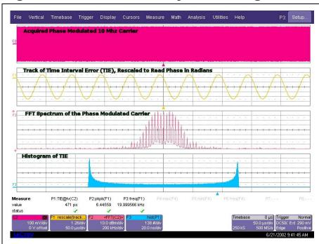
Figure 1 Analysis of a PM signal using the track of time interval error (TIE).
