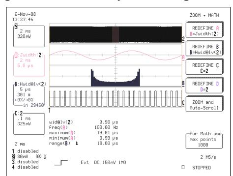
Figure 1 Analyzing a PWM waveform using JTA and histogram
