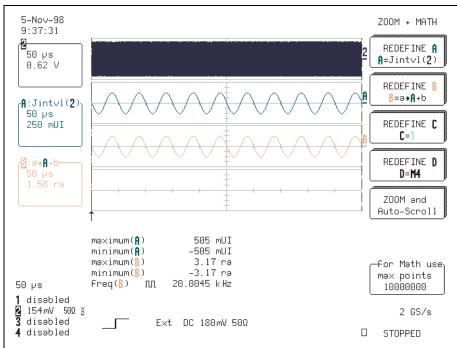
Figure 1 Analysis of a PM signal using both Time Interval Error (JIntvl) .
