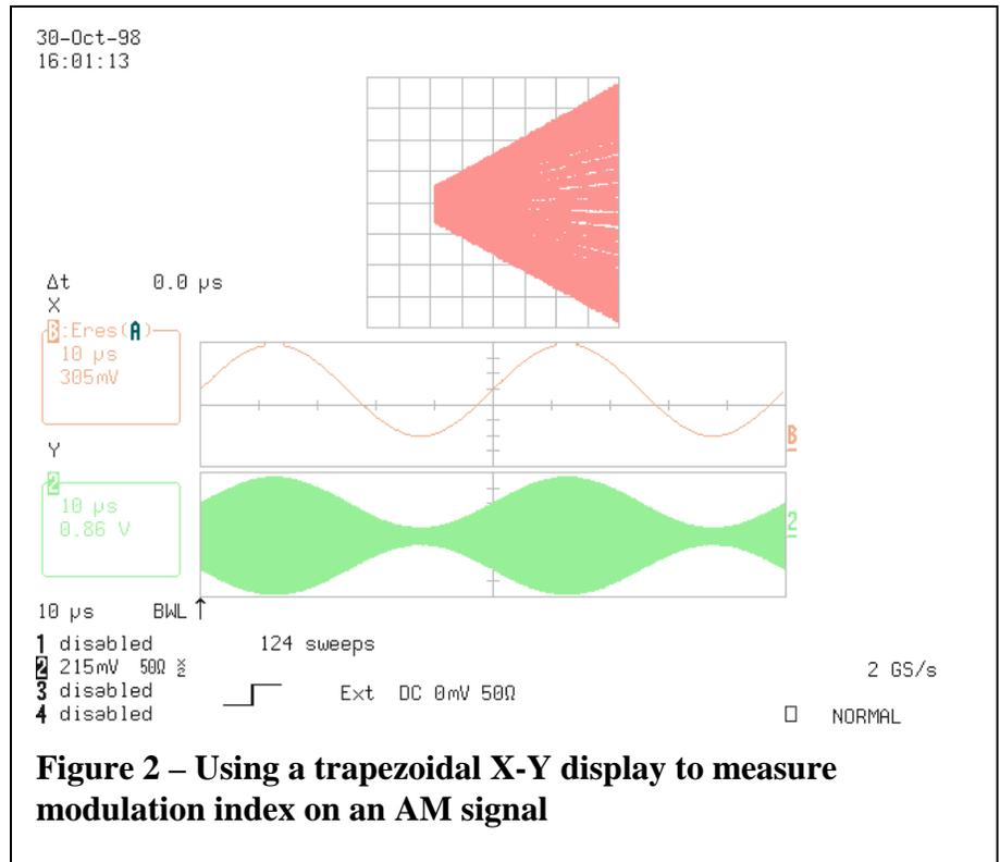
**Figure 2 – Using a trapezoidal X-Y display to measure modulation index on an AM signal**
