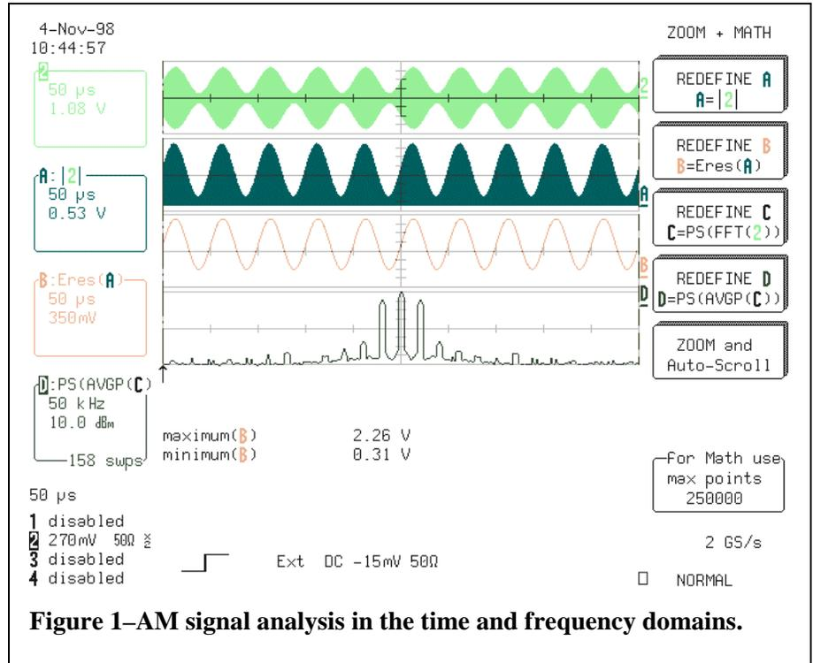
Figure 1—AM signal analysis in the time and frequency domains.
