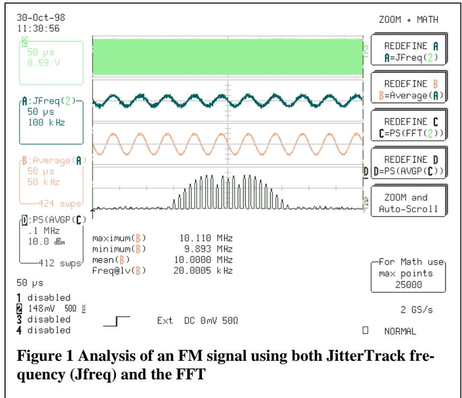
**Figure 1 Analysis of an FM signal using both JitterTrack frequency (Jfreq) and the FFT**
