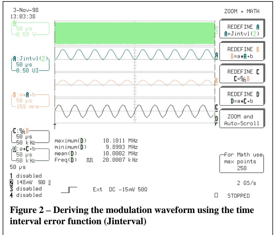
**Figure 2 – Deriving the modulation waveform using the time interval error function (Jinterval)**
