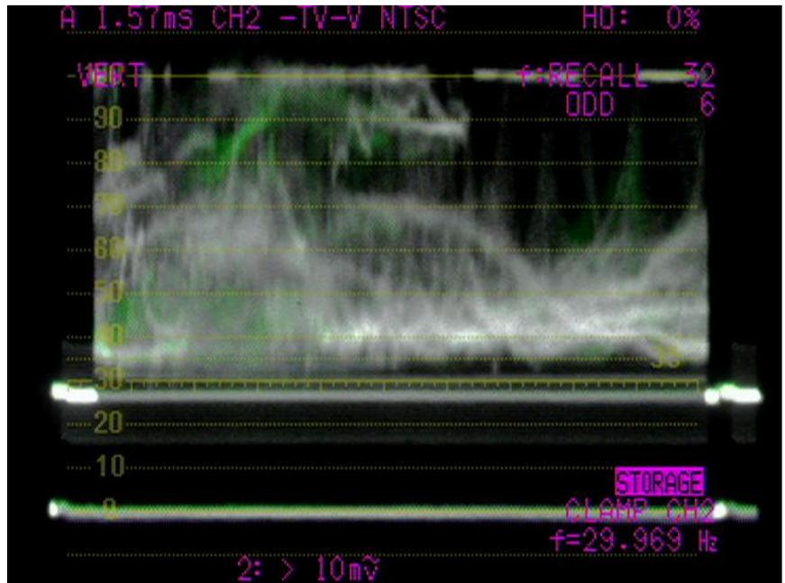
**Figure 3: Composite Video; TV Line Trigger (Odd Field Line Number 6) displaying one full video Frame. Dynamic changes in white, persistence fade in green.**
