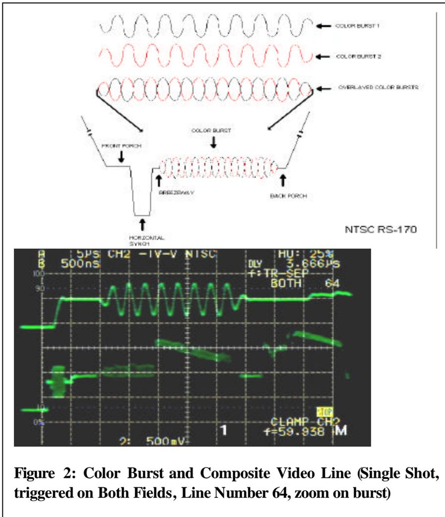
**Figure 2: Color Burst and Composite Video Line (Single Shot, triggered on Both Fields, Line Number 64, zoom on burst)**
