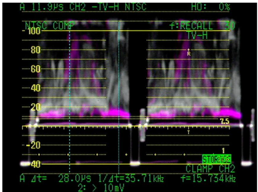
**Figure 4: Composite Video 2H with EIA scales displayed on LA354 with Storage enabled (violet is stored trace, white is live feed).**
