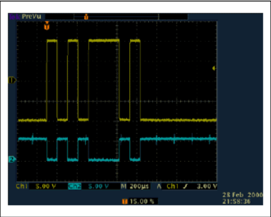
Figure 2. An RS-232 receiver accepts the bipolar input signal (top trace, CH1) and outputs an inverted TTL/
