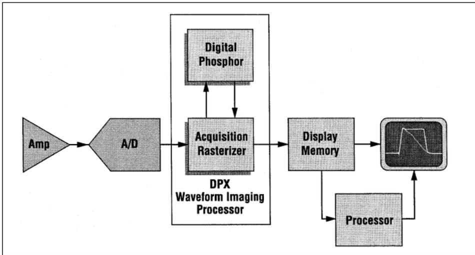
Figure 1. Tektronix DPO Architecture.
