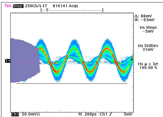
Figure 3. 1.85 GHz carrier and amplitude distribution of CDMA forward link, pilot only.
