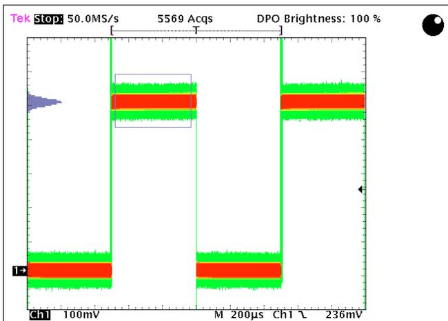
Figure 2. Histogram of noise on a square wave.
