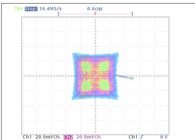
Figure 6. Unmodulated transient in demodulated CDMA forward link signal.
