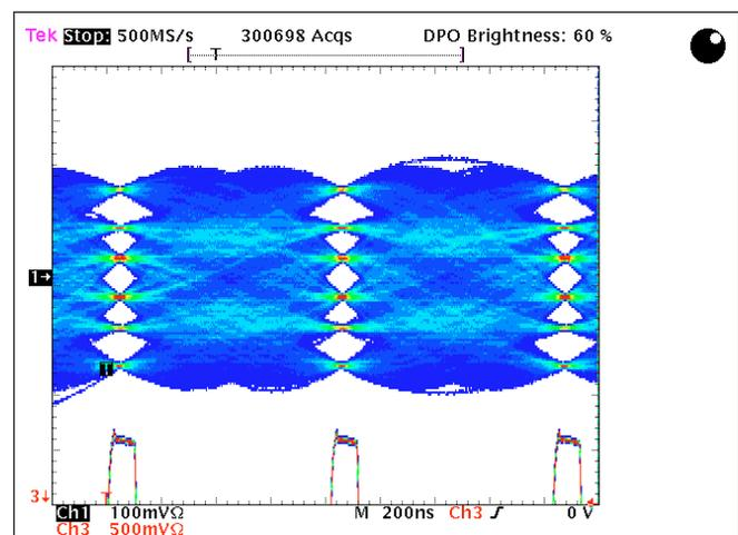
Figure 7. Eye Diagram and Z-axis trigger Synchronization for constellation display.
