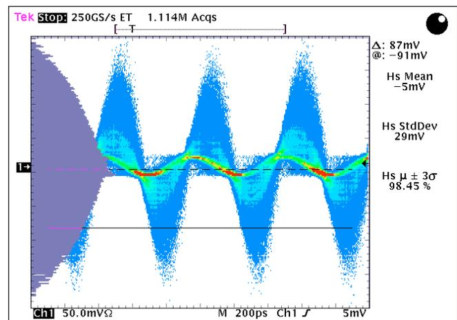
Figure 4. 1.85 GHz carrier and amplitude distribution, CDMA forward link. Walsh codes 0, 1, 8, 16, 24, 32, 40, 48, 56 at power levels per IS-97 recommendation.
