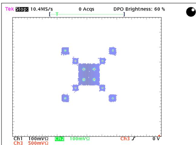
Figure 8. XYZ display of CDMA Forward Link.
