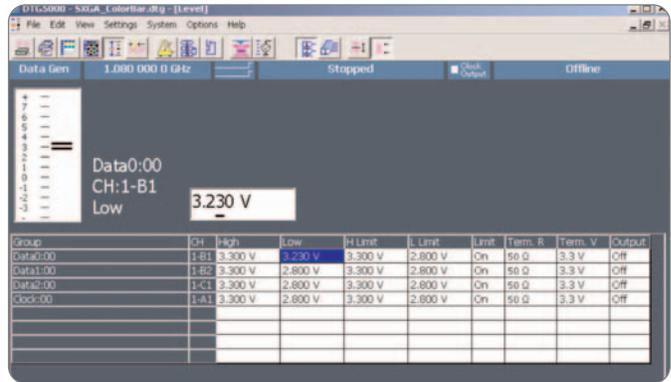
► Figure 11. Voltage Level setup menu in DTG5274
