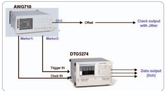
► **Figure 9.** Connecting an arbitrary waveform generator to increase range and variety of jitter.
