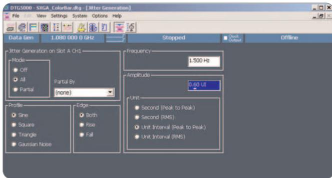
► **Figure 8.** Jitter setup menu in DTG5274.
