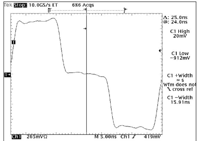
Figure 7. Duty cycle distortion measurement, negative pulse width.
