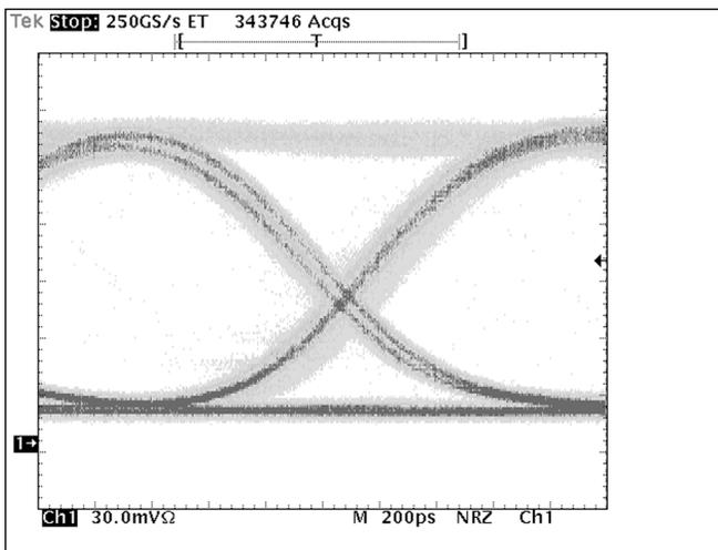
Figure 11. Color-graded eye crossing display.
