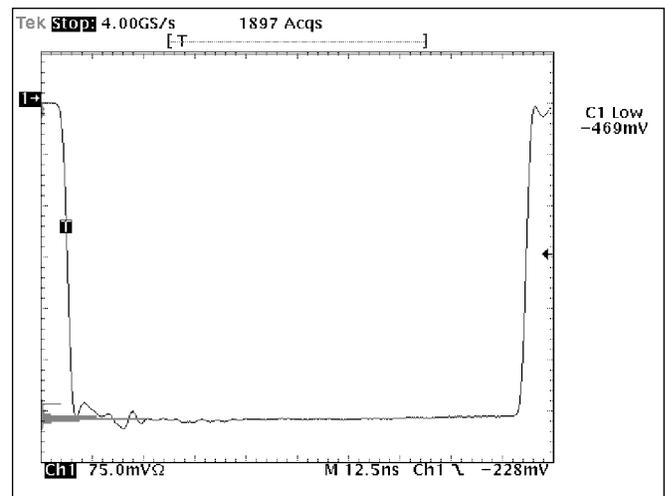
Figure 9. Negative MLT-3 pulse with low automatic measurement.
