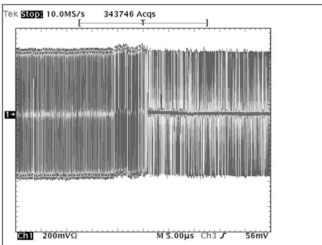
Figure 1. Baseline wander in a 100Base-TX signal observed with DPO.
