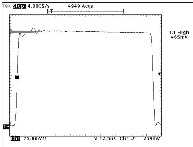
Figure 8. Positive MLT-3 pulse with high automatic measurement.
