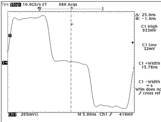
Figure 6. Duty cycle distortion measurement, positive pulse width.
