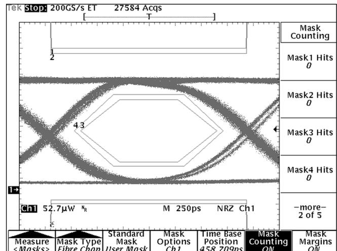
Figure 12. Eye diagram masks with 20% margin added.
