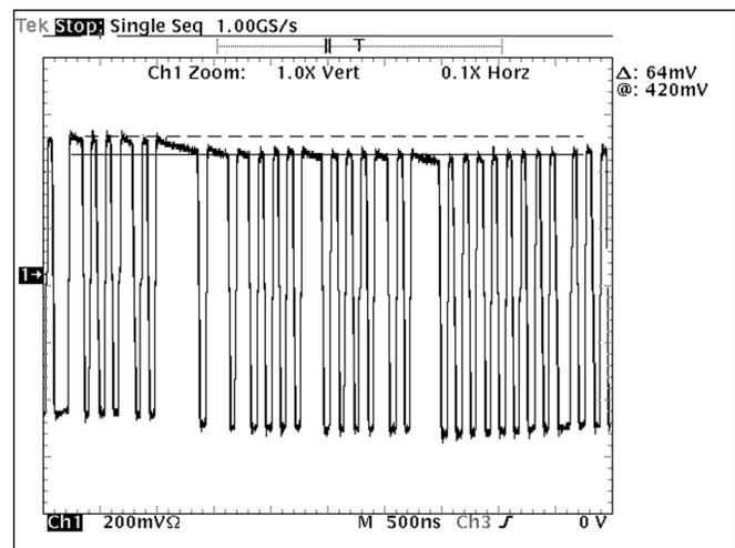
Figure 2. Baseline wander in a 100Base-TX frame at higher resolution.
