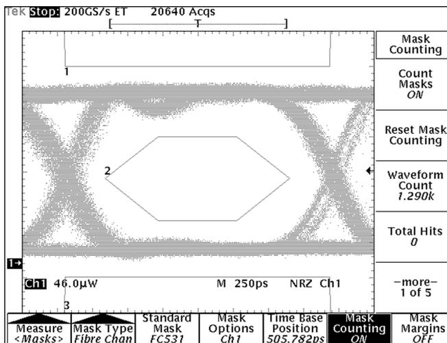
Figure 4. Fibre channel eye diagram mask test.
