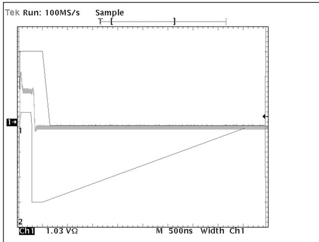
Figure 3. 10BaseT idle pulse mask.
