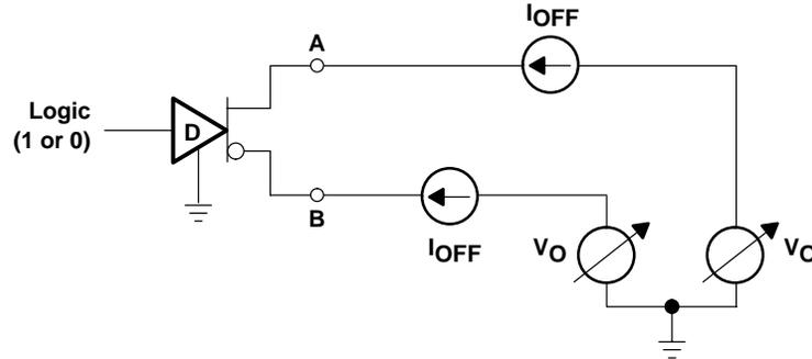
NOTE A:  $|I_{off}| \leq 100\ \mu\text{A}$  for  $-0.25 \leq V_O \leq 6\ \text{V}$
