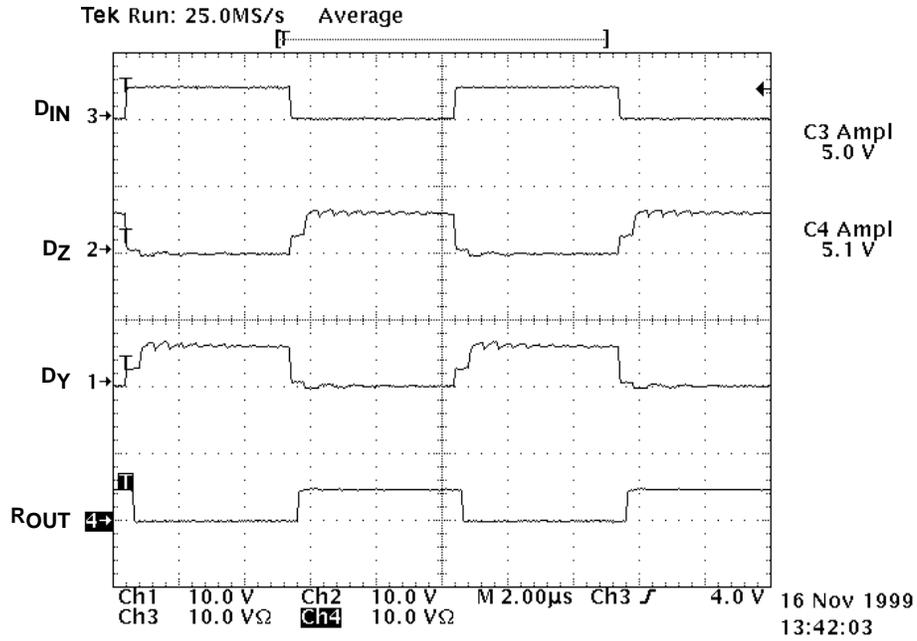
Figure 17. Differential Unterminated-Driver Output Waveforms
