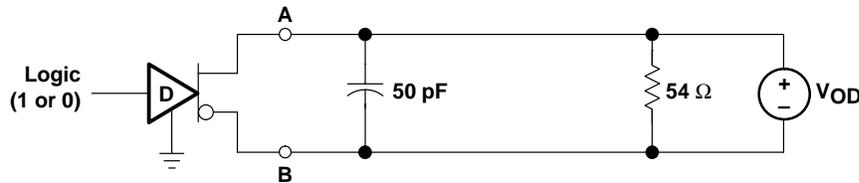
**Figure 15. Output-Signal Test Circuit**
