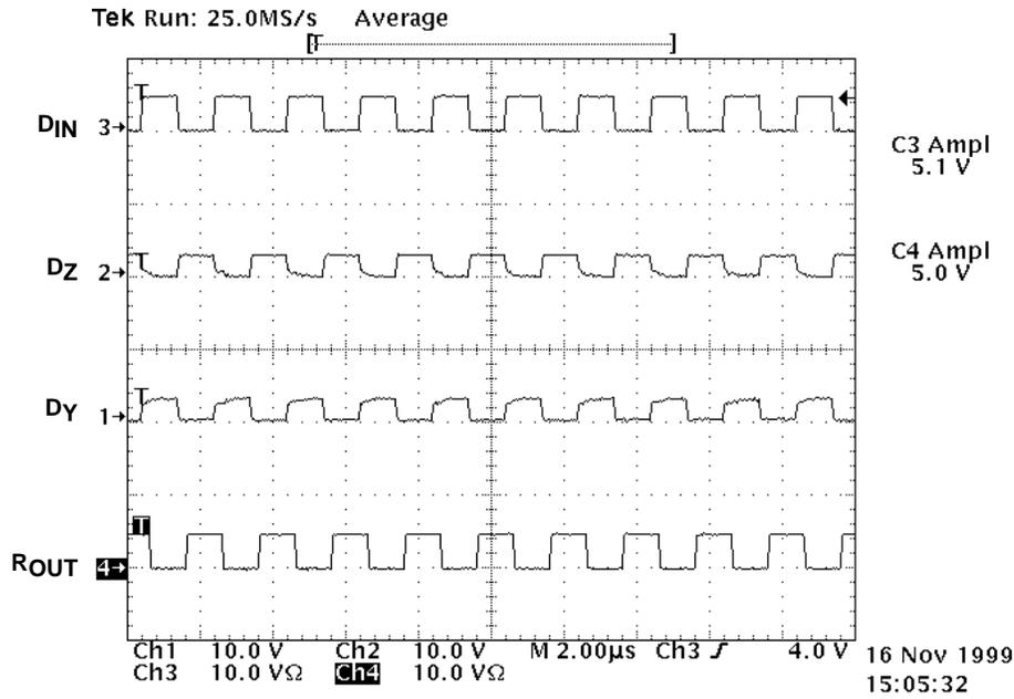
Figure 26. Differential Open-Line Fail-Safe-Terminated Driver Output Waveforms
