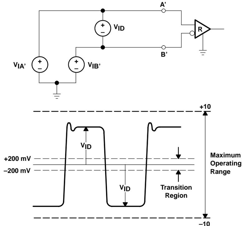
NOTE A:  $200\text{ mV} < |V_{ID}| < 10\text{ V}$
