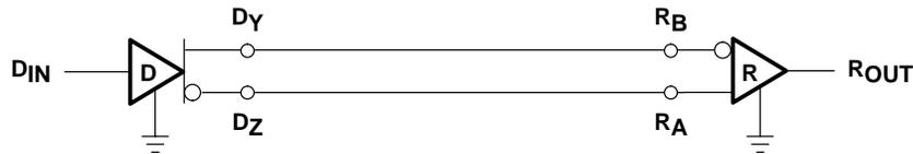
**Figure 16. Differential Unterminated Configuration**
