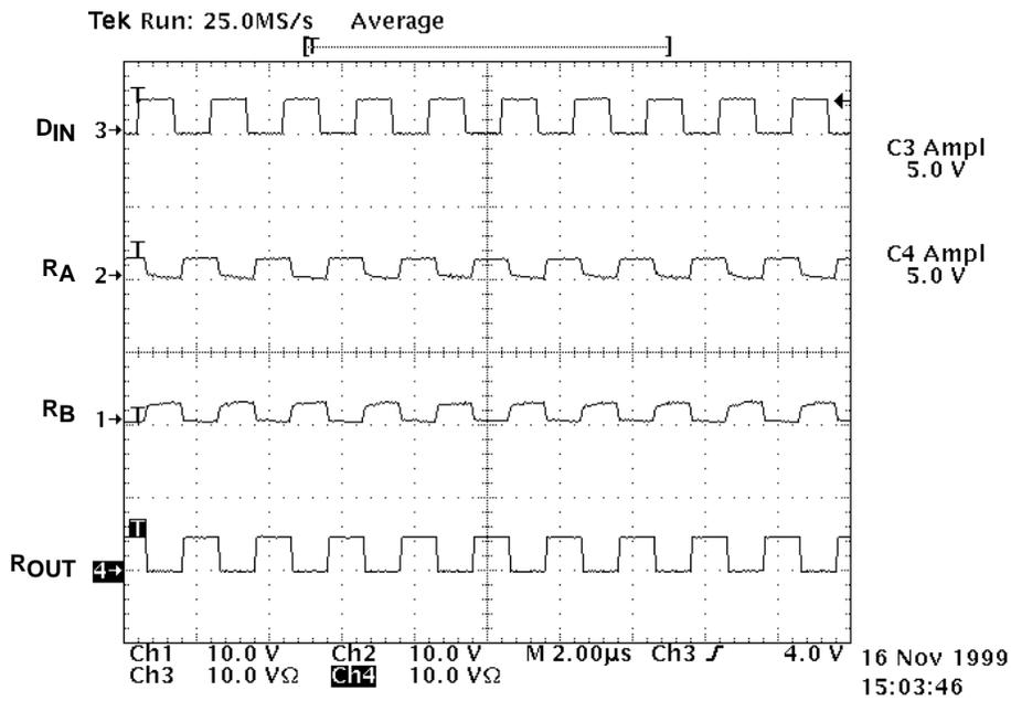
Figure 27. Differential Open-Line Fail-Safe-Terminated Receiver Input Waveforms
