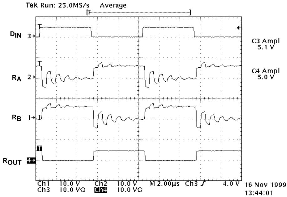
Figure 18. Differential Unterminated-Receiver Input Waveforms
