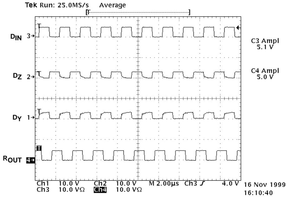
Figure 29. Differential Open-/Shorted-Line Fail-Safe-Terminated Driver Output Waveforms
