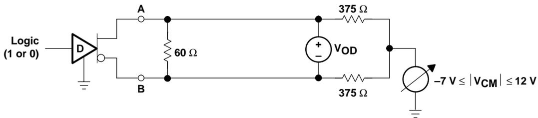
NOTE A:  $1.5 \text{ V} \leq |V_{OD}| \leq 5 \text{ V}$
