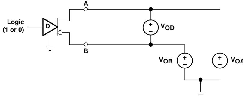
NOTES: A.  $1.5 \text{ V} \leq |V_{OD}| \leq 6 \text{ V}$
