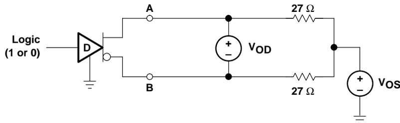
NOTES: A.  $1.5 \text{ V} \leq |V_{OD}| \leq 5 \text{ V}$ , and  $|\Delta V_{OD}| = \left| |V_{OD}| - \frac{|V_{OD}|}{2} \right| \leq 0.2 \text{ V}$
