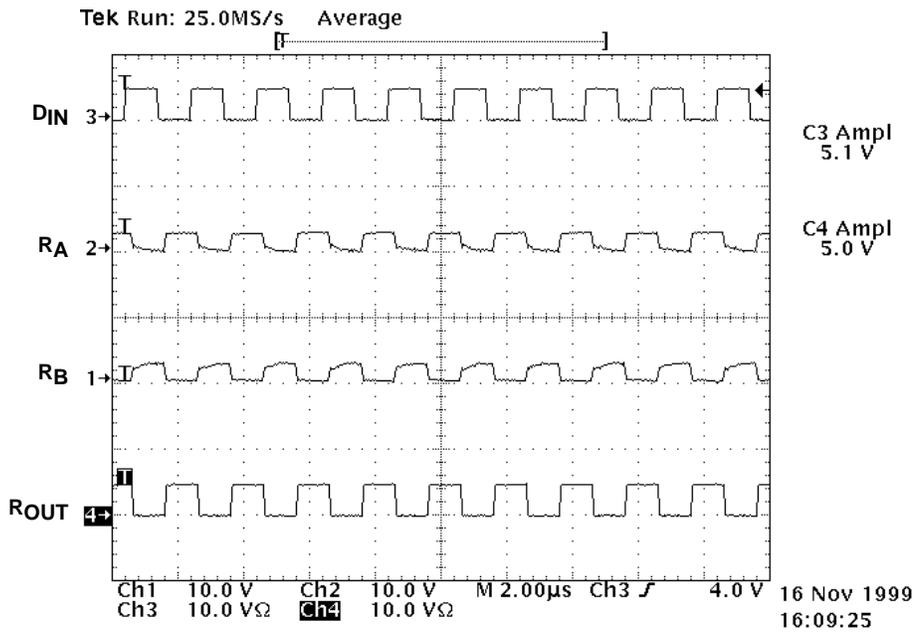
Figure 30. Differential Open-/Shorted-Line Fail-Safe-Terminated Receiver Input Waveforms
