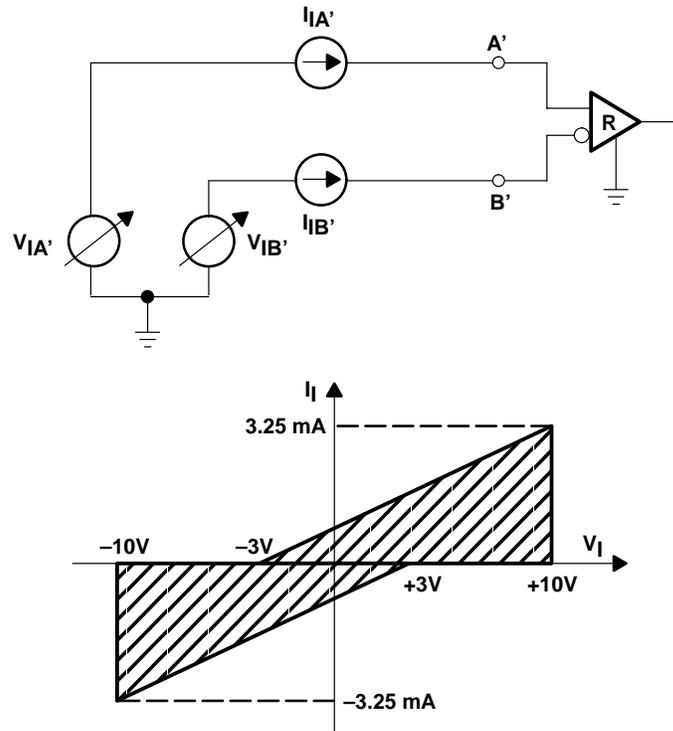
NOTE A:  $R = \Delta V / \Delta I = 13 \text{ V} / 3.25 \text{ mA} = 4 \text{ k}\Omega$
