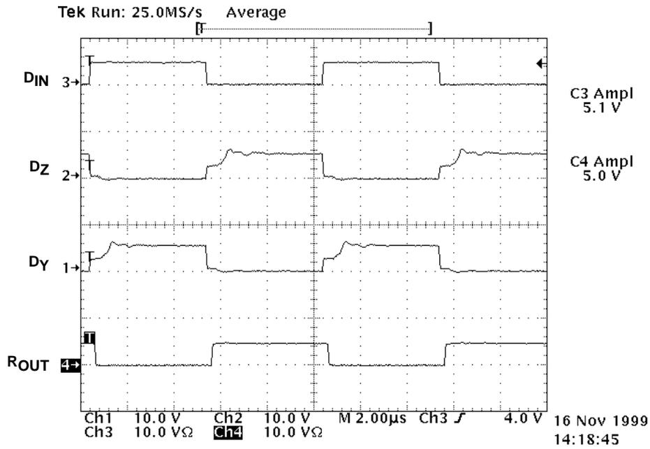
Figure 23. Differential AC-Terminated Driver Output Waveforms
