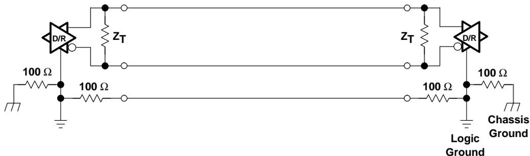
**Figure 32. Recommended Grounding Configuration**
