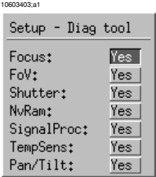
Figure 12.1 Setup – Diag tools: Press the navigation pad left/right for each test to include or exclude it from the diagnostic test.
