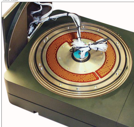
Figure 12.3 Exterior Housing Heaters Option, showing one of the foil heaters
