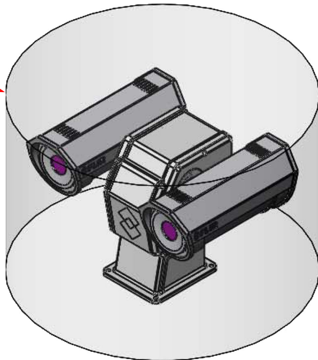
Figure 1-2: PT-Series Pan and Tilt Exclusion Zone
