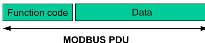
Figure 5: MODBUS Protocol Data Unit
