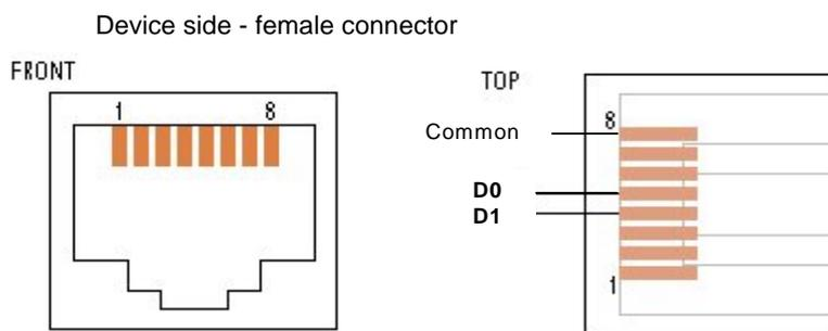
Figure 24: 2W- MODBUS on RJ45 connector ( required pin-out )
