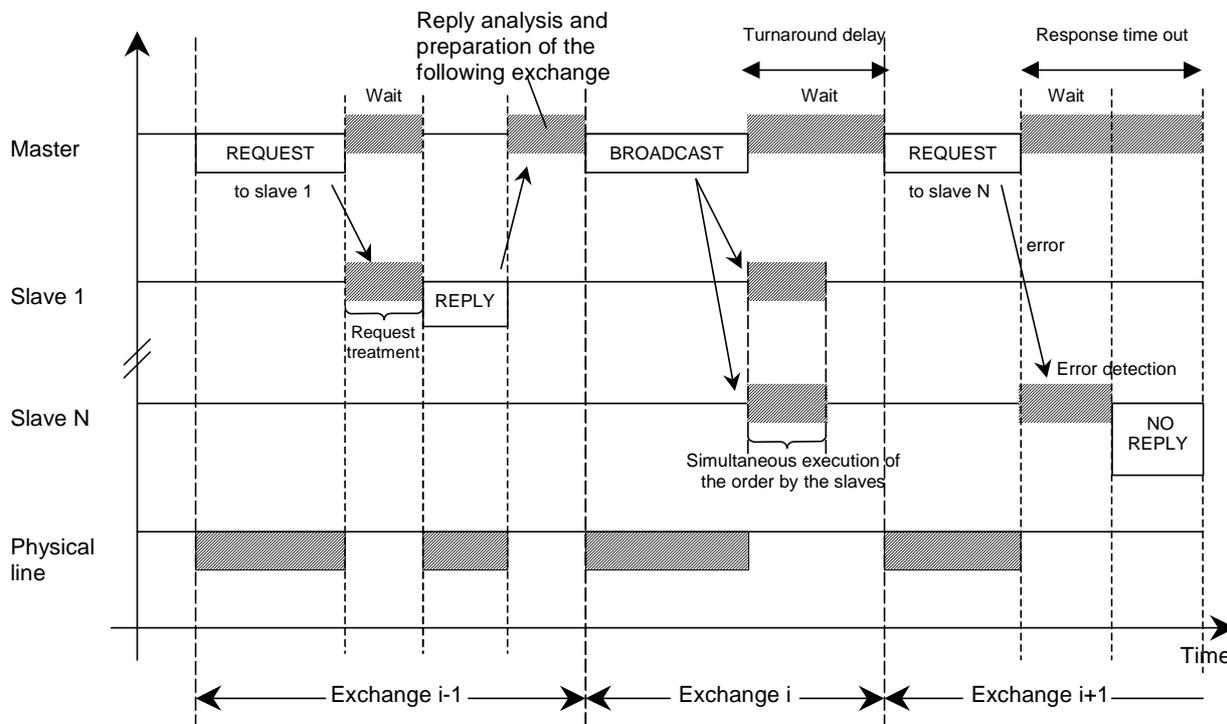
Figure 9: Master / Slave scenario time diagram
