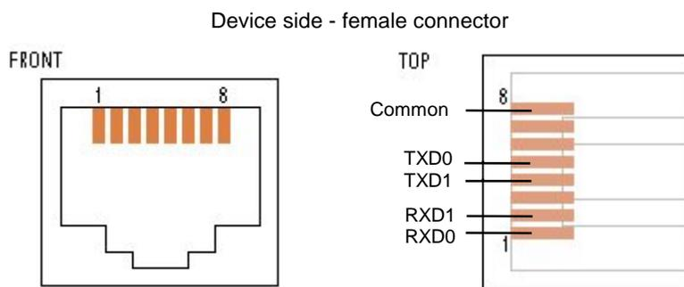
Figure 26: 4W- MODBUS on RJ45 connector ( required pin-out )
