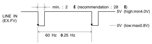
Signal Spec. of AC-Line Pulse (EX.FV)
