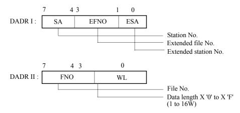
• The station number of each controlled station connected to the line is designated by 5 bits with ESA and SA as shown in the following figure.
