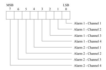
$\begin{array}{ccc} Alarm \ decision \ result \ ON \ : & Corresponding \ bit = 1 \\ OFF : & Corresponding \ bit = 0 \end{array}$
