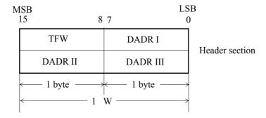
Elements of the header section are explained in units of byte as follows.
