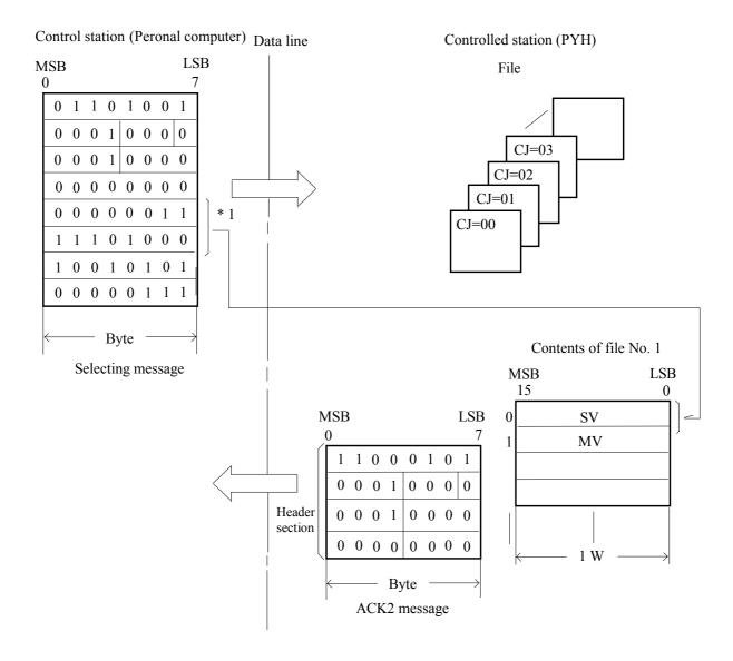
\* 1 SV is a % value to the measuring range, and 0 to 10000 corresponds to 0 to 100.00%. Since the SV is set to 100°C in the measuring range of 0° to 1000°C in this example, SV is 10%, that is, 1000 (X' 3E8') is stored into the file.
