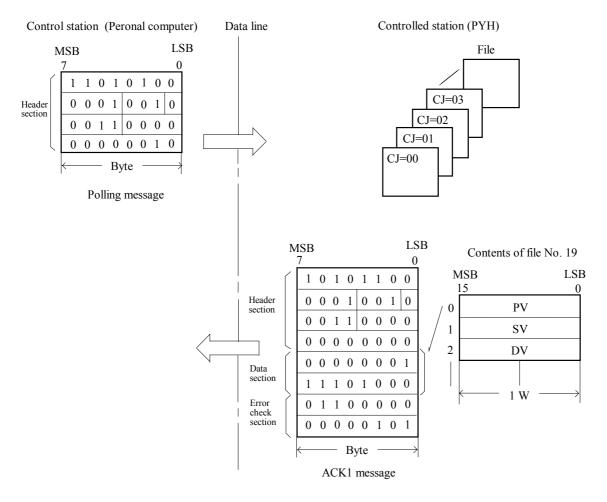
\*1 PV is a % value to the measuring range, and 0 to 10000 corresponds to 0 to 100.00%. Since PV is 100°C in the measuring range of 0° to 1000°C in this example, PV is 10%, that is, 1000 (X' 3E8') is stored into the file.
