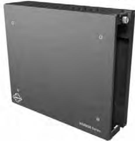
Up to four Endura® system modules can be installed when using the **WM5200-4U** wall mount kit. The base kit includes a wall bracket that can be mounted onto a wall in any orientation and a module sleeve with cover plate. The **WM5200-4UEXP** expansion kit includes an additional module sleeve. Three expansion kits can be attached to the base kit for a maximum of four module sleeves.
