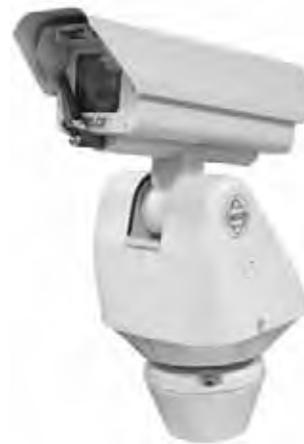
A powder-coated, aluminum construction makes the **ES30PC** and **ES31PC** ideal for either indoor or outdoor applications. The system has an absolute operating temperature range of  $-50^{\circ}$  to  $140^{\circ}$ F ( $-45^{\circ}$  to  $50^{\circ}$ C). Within two hours after power-up, the entire unit can de-ice and be operational from a temperature of  $-13^{\circ}$ F ( $-25^{\circ}$ C).
