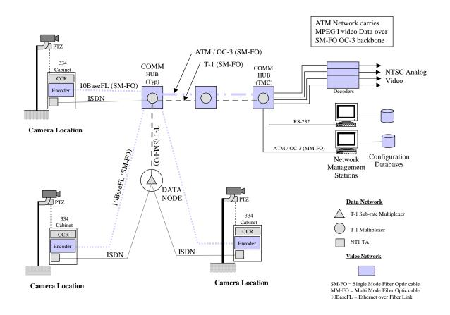
Figure 1. District 11 CCTV architecture – field to TMC.
