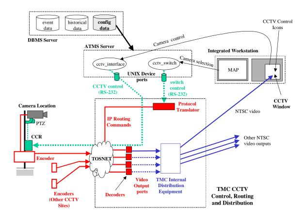
Figure 3. Advanced Traffic Management System (ATMS) CCTV control software.
