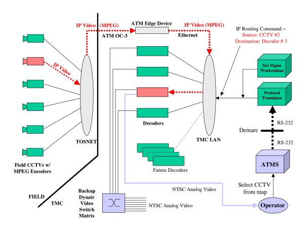
Figure 2. Internal TMC data conversion (ATM-to-Ethernet and digital-to-analog)
