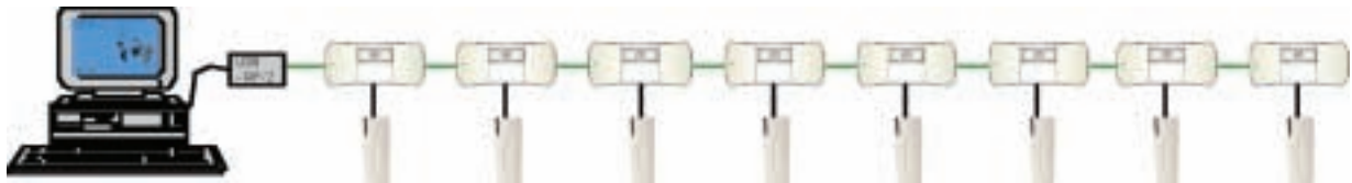
DC800 Door Controllers networked together using Entro Lite software and the USB-RIF/2 Interface
