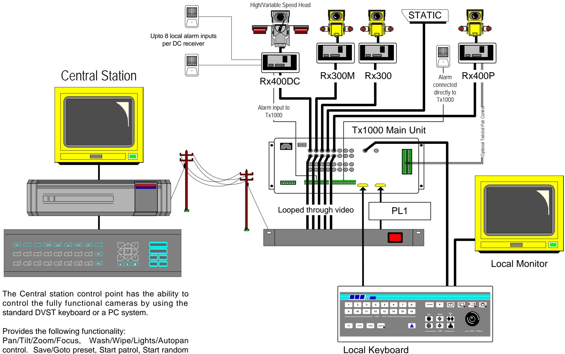
The Central station control point has the ability to control the fully functional cameras by using the standard DVST keyboard or a PC system.
