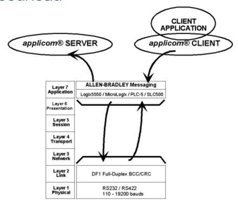
Several protocol configurations are allowed with the **Allen-Bradley** interface module and the **applicom**® card:
