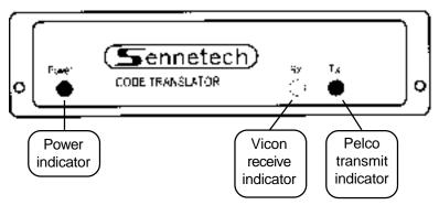
The receive indicator should flash when Vicon code is present on the input. If the code is a camera control command for a camera in the address window, the transmit indicator should flash when the converted Pelco command is sent. Vicon systems "poll" the cameras periodically so the receive indicator will probably flash even when no camera is being controlled.
