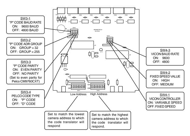
The code translator will appear as a group of cameras to the controller. To prevent interference between the responses from the code translator and any Vicon cameras in the system, set the switches to include only the Pelco camera addresses.
