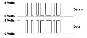
As can be seen by the above illustration, or as viewed on an oscilloscope, the data patterns for both the positive and negative sides of the line are equal but opposite in polarity with respect to ground.
