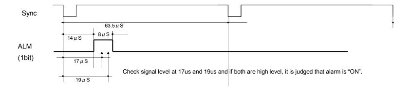
Fig. 2 : Alarm bit horizontal timing chart
