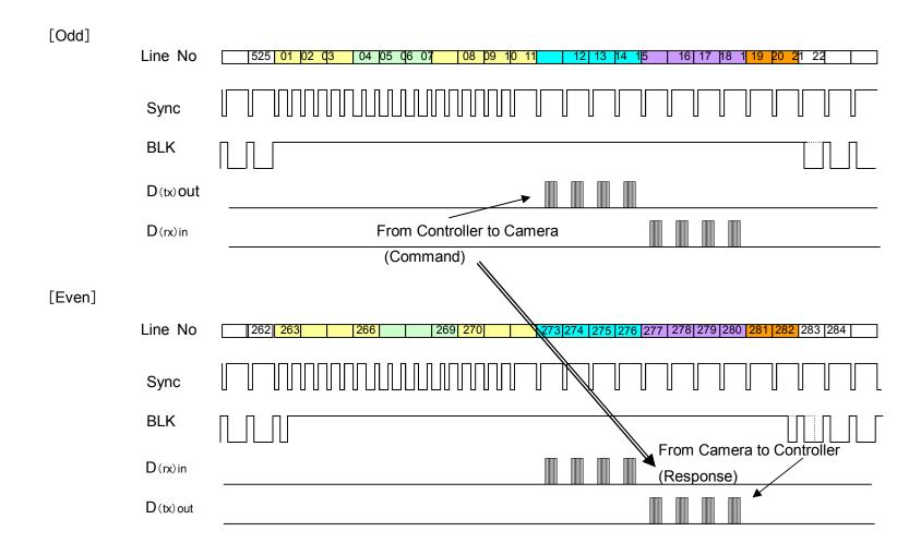
Fig.1-1 Command – response timing chart
