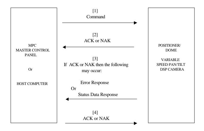
FIGURE 1. TYPICAL COMMUNICATION HANDSHAKE PROTOCOL
