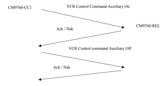
If an auxiliary is programmed to be a latching auxiliary, the CM9760-CC1 still sends the command two times. Once when the key is pressed and once when the key is released. If the relay is being turned on the CM9760-CC1 sends the on command twice. If the relay is being turned off, the CM9760-CC1 will send the off command twice.
